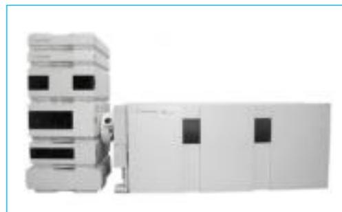
*Spectro possess LC-MS/MS to carry out testing of mycotoxins and pesticides residue in different food and feed products.*
