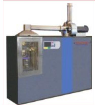
*Cone Calorimeter - ISO 5660 & ASTM E1354*
